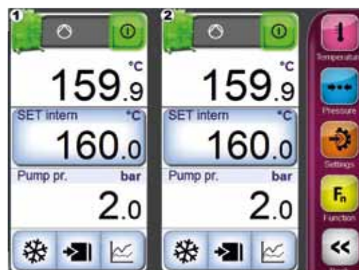
TEMPRO plus D Micro dual zone unit: display of both circuits on the touch-screen
